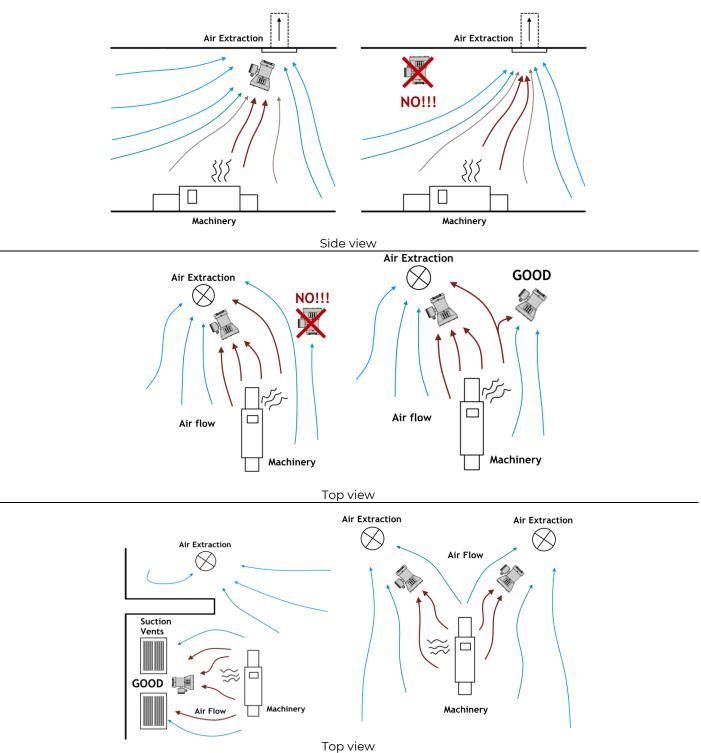
It is mandatory checking the air flow in the room where the OMD must be installed in order to identify the best installation point for measuring the Oil Mist.
